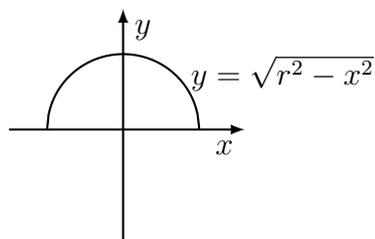
$$\begin{aligned} S &= 2\pi \int_{-r}^r \sqrt{r^2 - x^2} \sqrt{1 + \left(\frac{-2x}{2\sqrt{r^2 - x^2}}\right)^2} dx \\ &= 4\pi \int_0^r \sqrt{r^2 - x^2} \frac{|r|}{\sqrt{r^2 - x^2}} dx = 4\pi r [x]_0^r = 4\pi r^2 \end{aligned}$$
