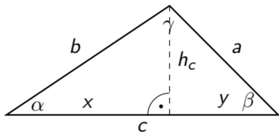
$$\begin{aligned} a^2 &= h_c^2 + y^2 = h_c^2 + (c - x)^2 = (b \sin \alpha)^2 + (c - b \cos \alpha)^2 \\ &= b^2 \sin^2 \alpha + c^2 - 2bc \cos \alpha + b^2 \cos^2 \alpha \\ &= b^2 \underbrace{(\sin^2 \alpha + \cos^2 \alpha)}_1 + c^2 - 2bc \cos \alpha \end{aligned}$$
