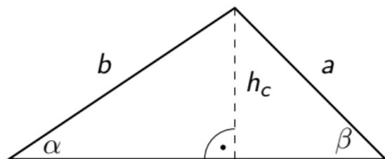
$$\sin \alpha = \frac{h_c}{b} \quad \Rightarrow \quad h_c = b \cdot \sin \alpha \quad (1)$$
