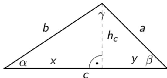
$$\begin{aligned} a^2 &= h_c^2 + y^2 = h_c^2 + (c - x)^2 = (b \sin \alpha)^2 + (c - b \cos \alpha)^2 \\ &= b^2 \sin^2 \alpha + c^2 - 2bc \cos \alpha + b^2 \cos^2 \alpha \end{aligned}$$
